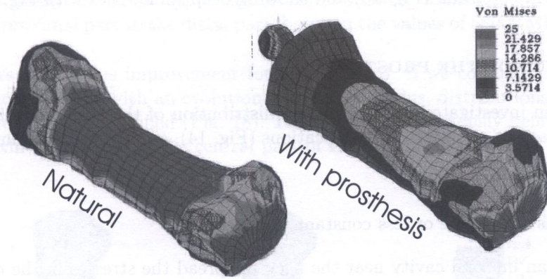
Fig. 10. Mises stresses from finite elements models
